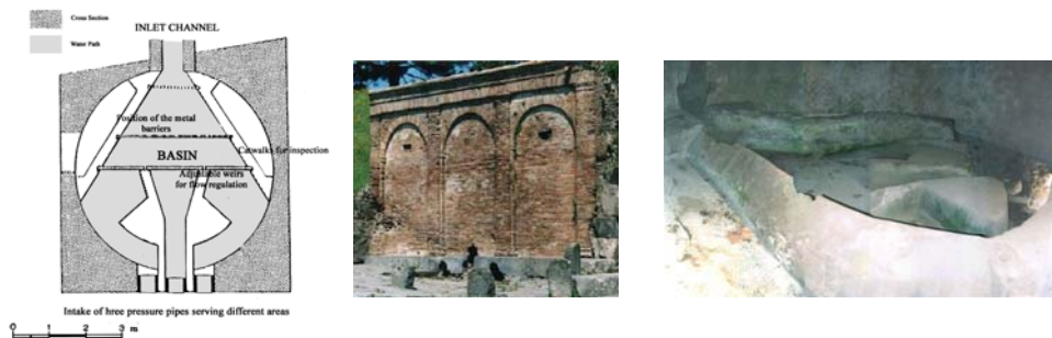
Figure 10. Castellum Divisorium in Pompeii: Plan, S-E Facade, View of the interior catwalks and partitioning masonry walls.
